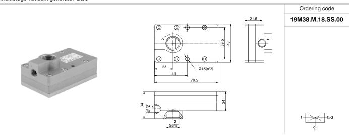
Compact generators comprising a number of modules as a function of the desired performance allow high-suction capacity with low consumption and other degrees of vacuum; as a function of the modules (nozzles 2-4-6-8) used, offer exactly the right performance for the most varied of industrial applications. They ensure a low level of noise thanks to the sound-absorbent material inside of them.
