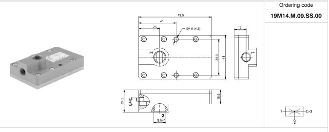
Compact generators comprising a number of modules as a function of the desired performance allow high-suction capacity with low consumption and other degrees of vacuum; as a function of the modules (nozzles 2-4-6-8) used, offer exactly the right performance for the most varied of industrial applications. They ensure a low level of noise thanks to the sound-absorbent material inside of them.
